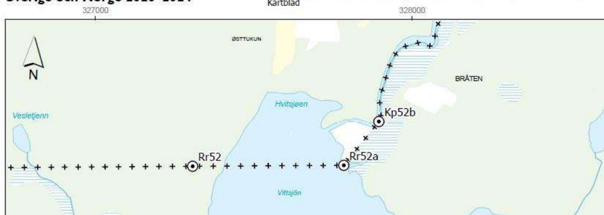
Figure 7: The boundary line goes as a straight line from boundary marker no 52 to 52a where a new stone cairn has been erected and then as a straight line to a point defined by coordinates (52b) in a creek, which the boundary line from there on follows northwards.
