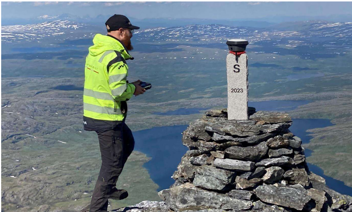
Figure 6: A small stone cairn as a boundary marker that do not define the boundary has been erected on the highest point along the boundary (1752 metres above mean sea level), here surveyed with network RTK by Swedish field engineer Karl Tirén.
