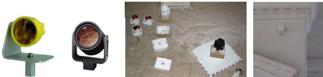
Figure 12: Leica-Prism GPR112 ( < 1\text{mm} ) and GPR1 ( \ll 1\text{mm} ), varnished and installed
