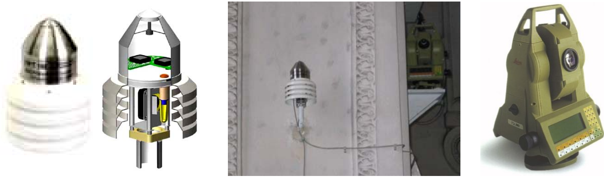
Figure 11: Sensors: Reinhardt DMT IMV (left) and Leica-TCA2003 (right)
