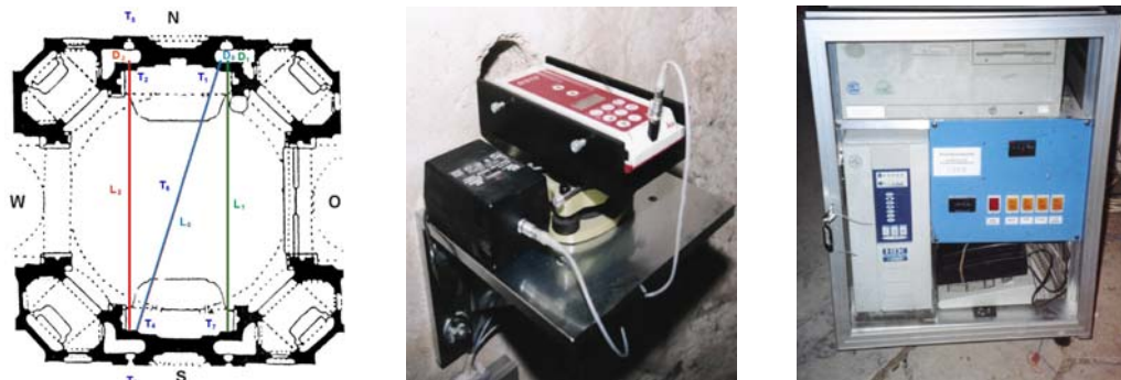
Figure 6: Convergence measurements with “Distos” in the benedictine monastery Rott a. Inn
