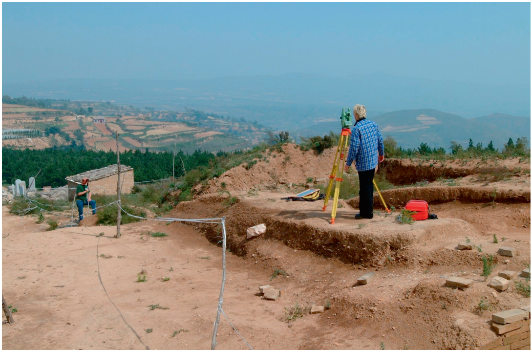
Fig. 1: Recording of archaeological findings using tachaeometry
