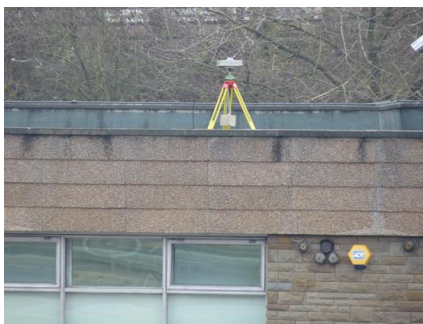
Figure 3. The principal reference GNSS antenna located upon an adjacent building to the bridge.
