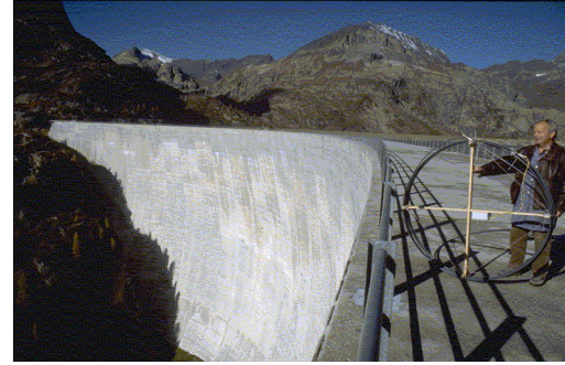
Figure 7 – A long sensor on its transporting spool
