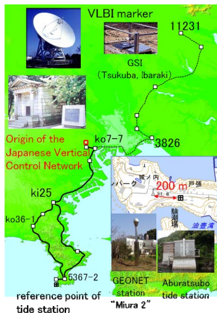
Fig. 7 Leveling route used in calculation of elevation of the Origin of the Japanese Vertical Control Network
