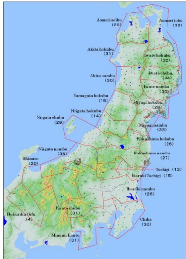
Fig. 8 Area map showing where triangulation stations for precise geodetic surveys and triangulation stations were resurveyed after the Tohoku Earthquake
