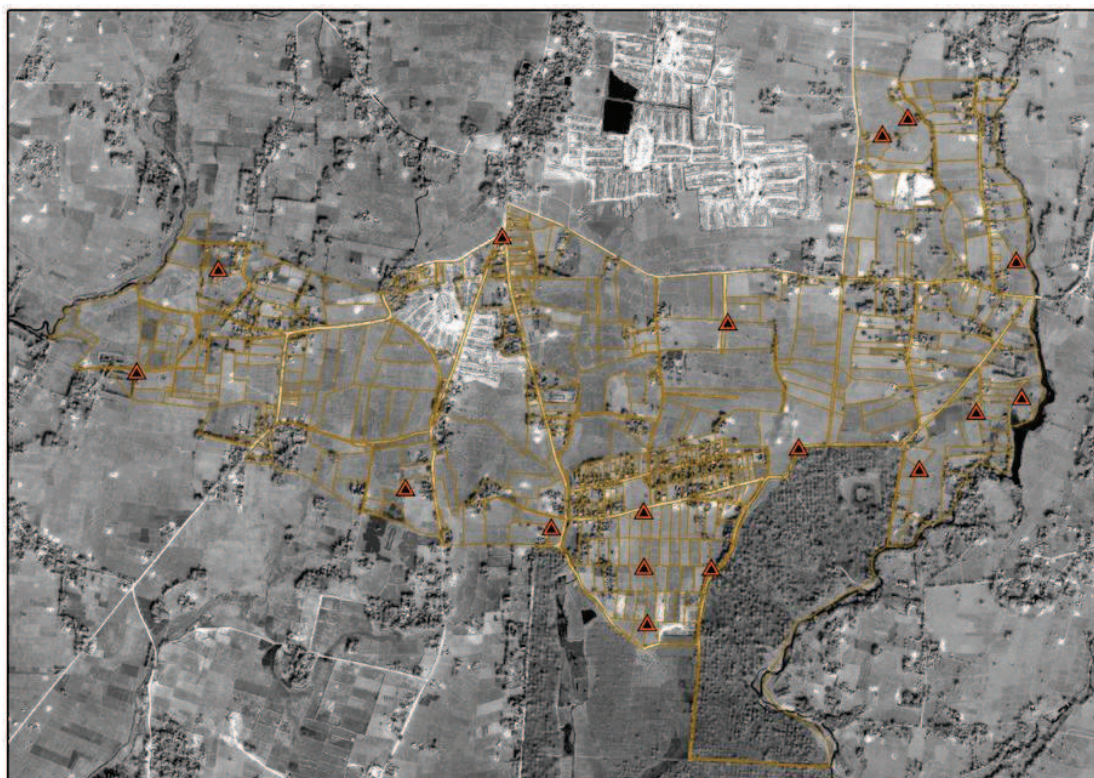
Fig. 4: Distribution of Control points for orientation of satellite Image
