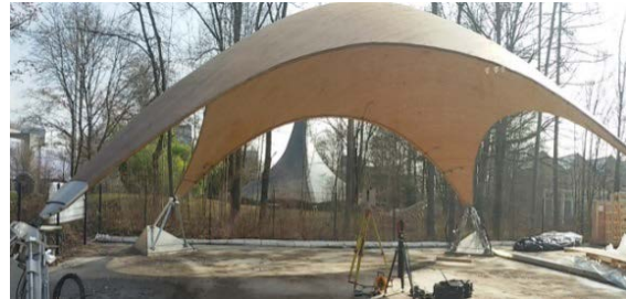
Fig 6 HDS 7000 laser scanner position
