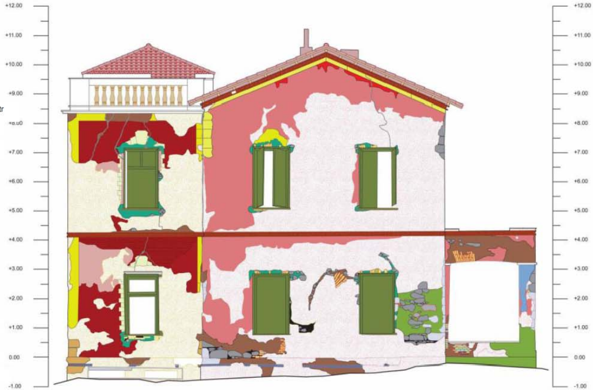
Thematic Map of Building Material and Decay Patterns in the South Façade of the Building
