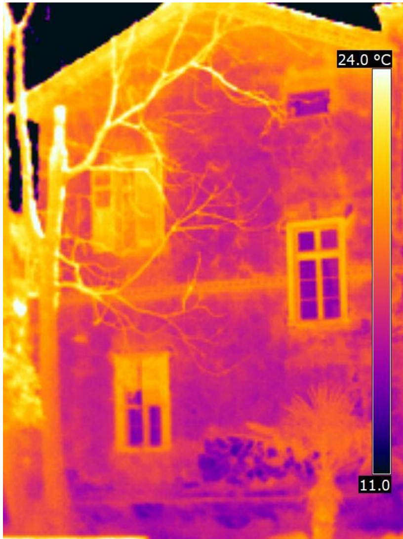
North Façade, Thermal mapping of the façade – indications of different construction phases
