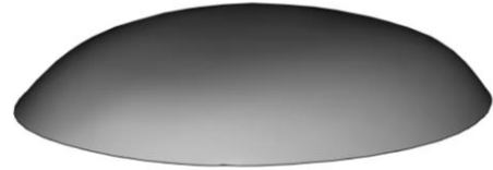
Figure 8: 12x12 B-Spline surface used as geometry for the FEM
