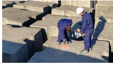
Figure 10 – Coordinating a GCP. The greenish colour of the surface of the blocks is due to slime
