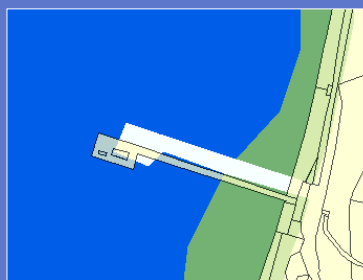
Problem when incorrect imagery scale is used to derive mapping: Zooming in to 1:30,000 mapping generated from imagery shows errors when compared to 1:2,500 vector mapping.
