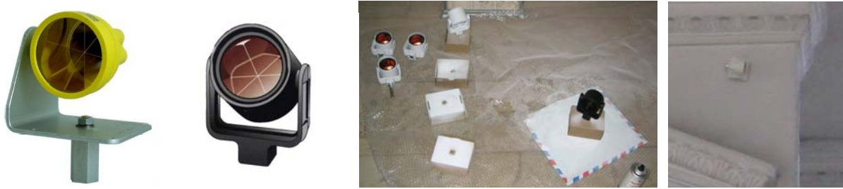
Figure 3: Leica-Prism GPR112 ( <1mm ) and GPR1 ( <<1mm ), varnished and installed
