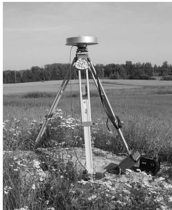
Figure 2. Observations were collected with dual frequency receivers and choke ring antennas using tripods.
