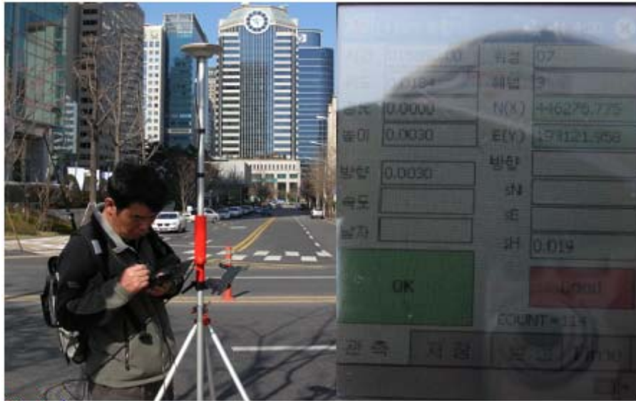
<Figure 4> GPS surveying data received accurately on PDA
