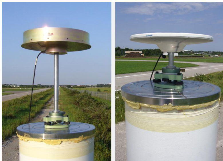
Fig. 4: Pillars and antenna mounting
