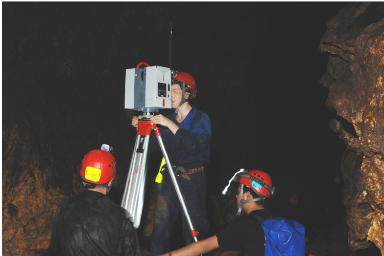
Fig. 6: TLS measurement in Gua Seropan
