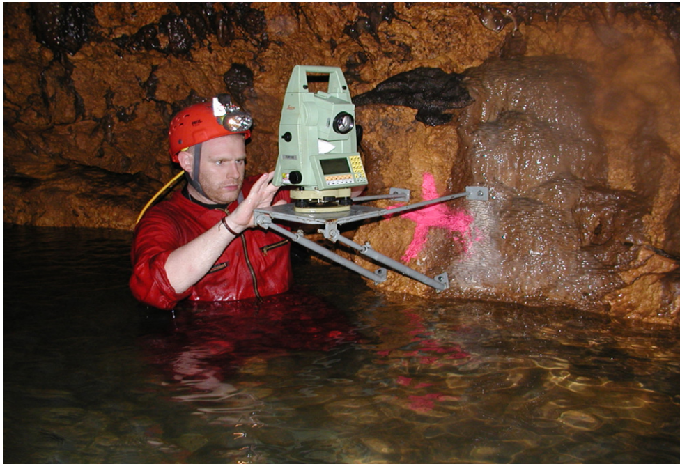
Fig.2: Polygon measurement using consoles in a lake area
