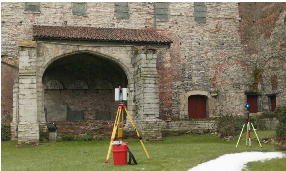
Figure 1: Laser scanner setup (Leica HDS 6100) at ‘Sint-Baafs Abbey’ (Gent, Belgium) (2010)
