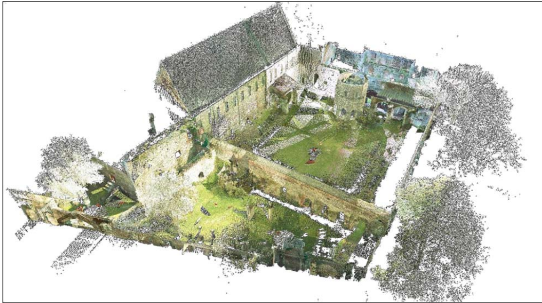
Figure 3: RGB colored point cloud of 'Sint-Baafs Abbey' derived from measurements with Leica ScanStation2 (own research, 2009)
