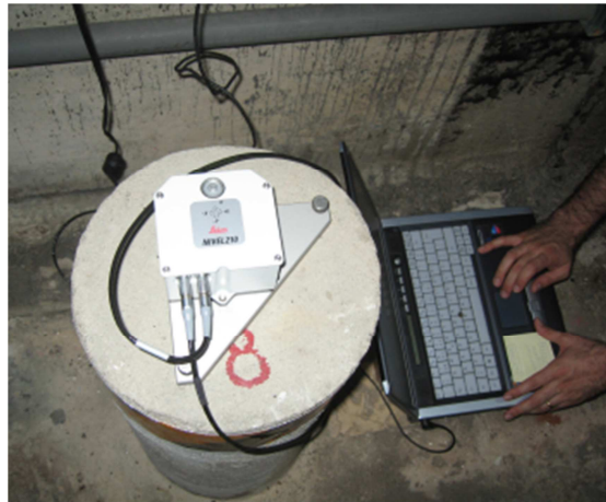
Figure 15 – Inclinometer setting up: computer
