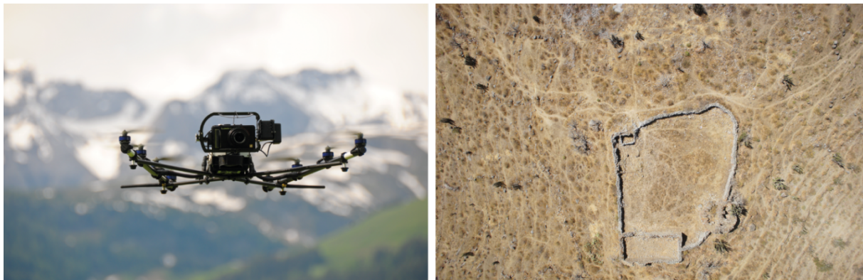
Figure 3: A Falcon 8 UAV as distributed by Ascending Technologies (left) 2 . An image of the site Santa Maria acquired with a ground pixel size of 2.5 cm, taken from 60 m above ground (right).
