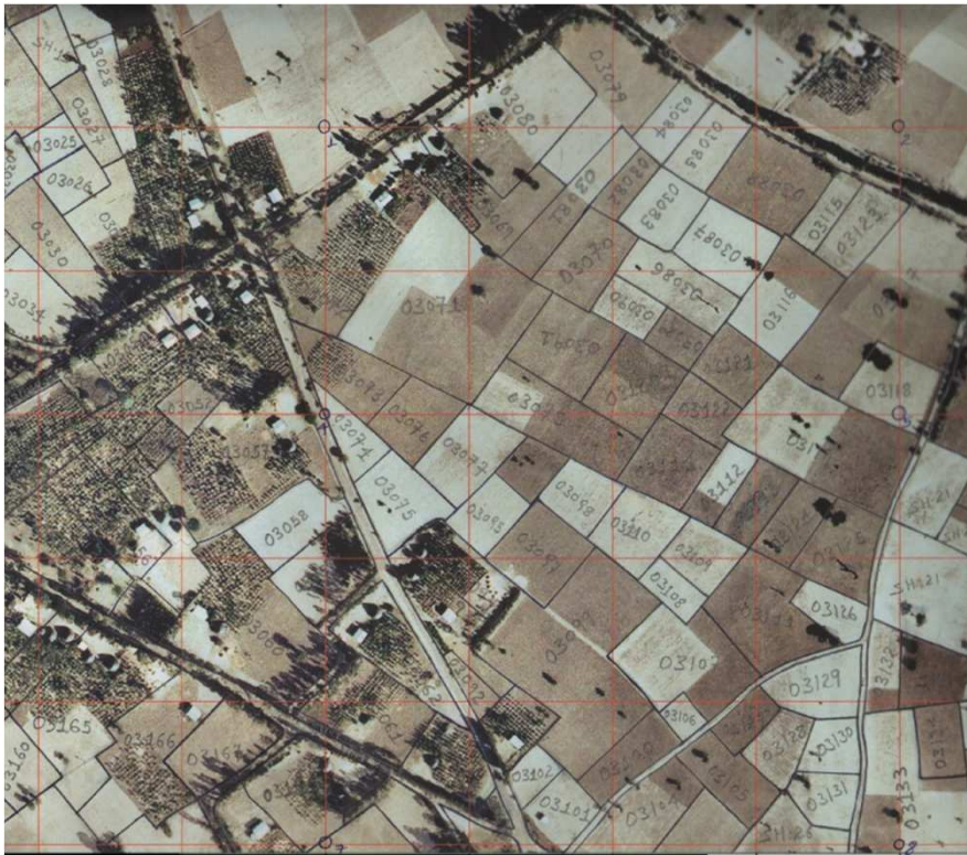
Orthophoto used as a field work map sheet with a georeferenced grid. The map shows the delineated parcel boundaries and parcel identification numbers.
