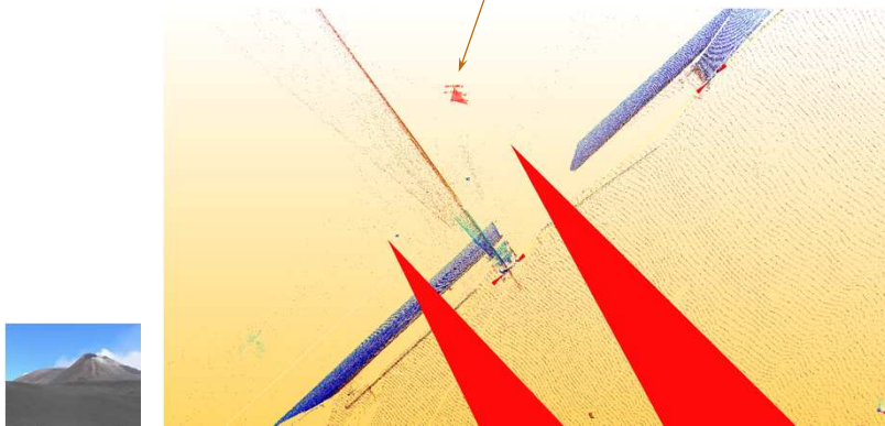
Fig. 4 The deviation in the position of the beam's axis, highlighted as triangle
