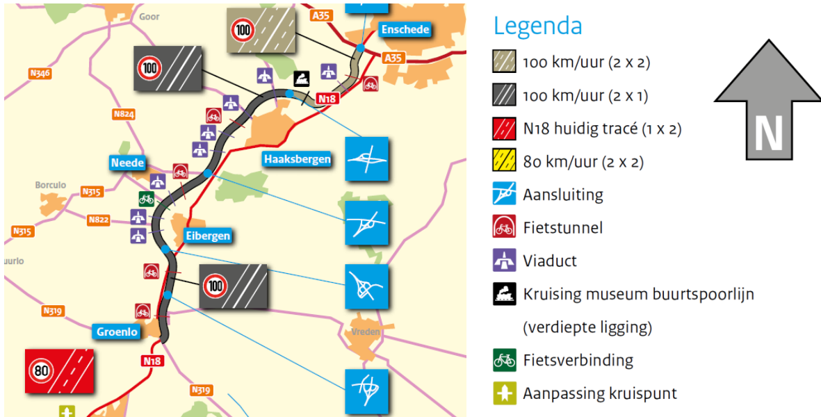
Figure 1 Road design for the bypass (Rijkswaterstaat, 2016)
