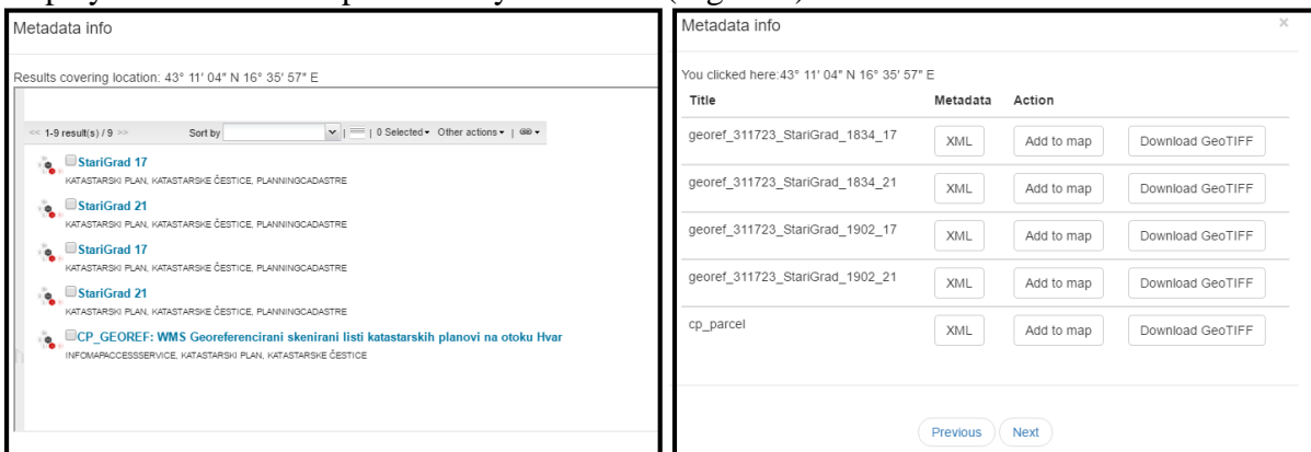
Figure 6. Result lists: left native GeoNetwork representation, right parsed from standard CSW GetRecords response XML
