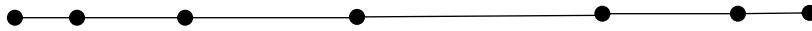
Figure 3 Segment points are dense on both ends and sparse in the middle of the baseline
