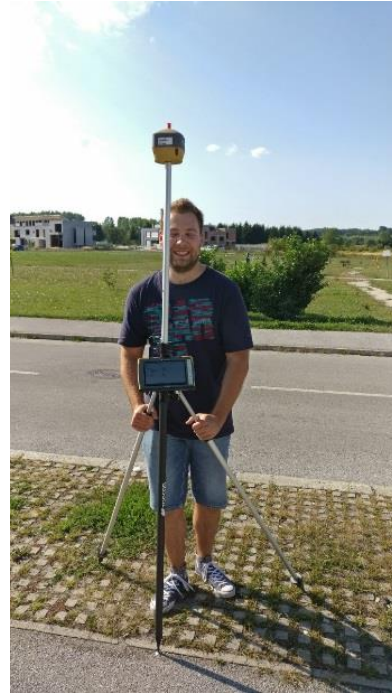
Figure 10. Rover GNSS receiver Topcon Hiper HR on the ranging pole with a bipod support
