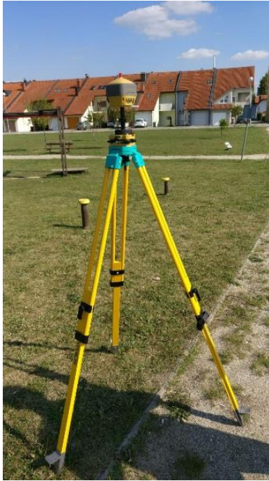
Figure 9. Base GNSS receiver Topcon Hiper HR on a tripod
