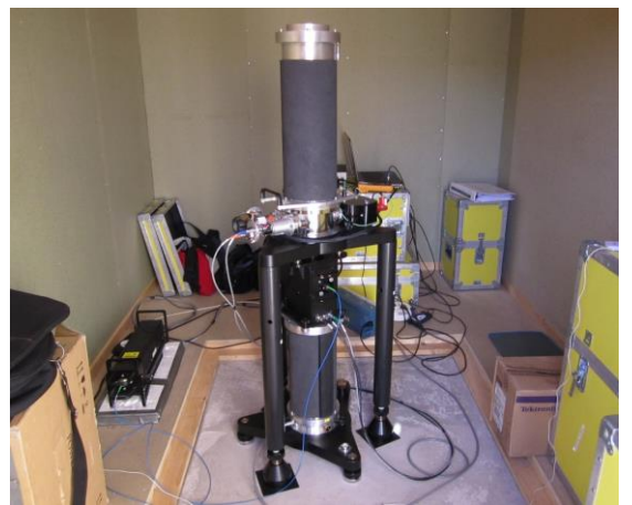
Figure 4. The Lantmäteriet FG5-233 absolute gravimeter, measuring at Smögen AA, Sweden.
