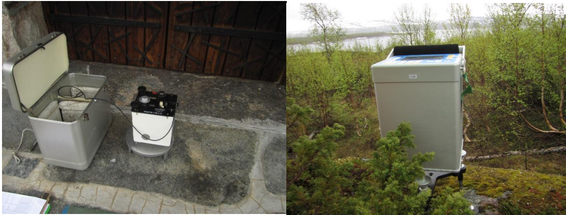
Figure 6: Left Relative observations with the LaCoste & Romberg G54 in Karesuando AA. Right with the Scintrex CG5-1184 in Umbukta A, Sweden.
