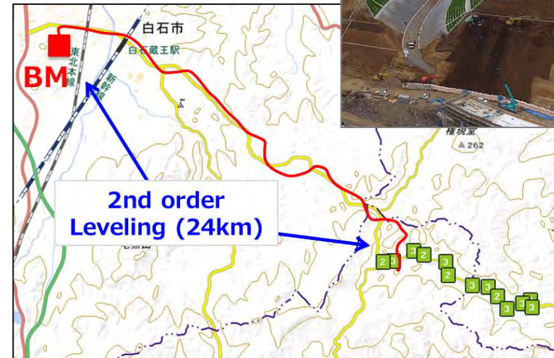
Altitude determination for road reconstruction
