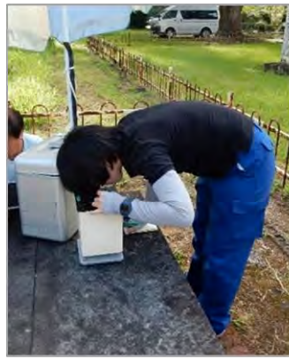
Relative Gravity Measurement (La-Coste)
