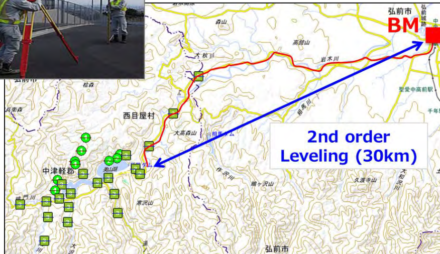
Altitude determination for dam construction
