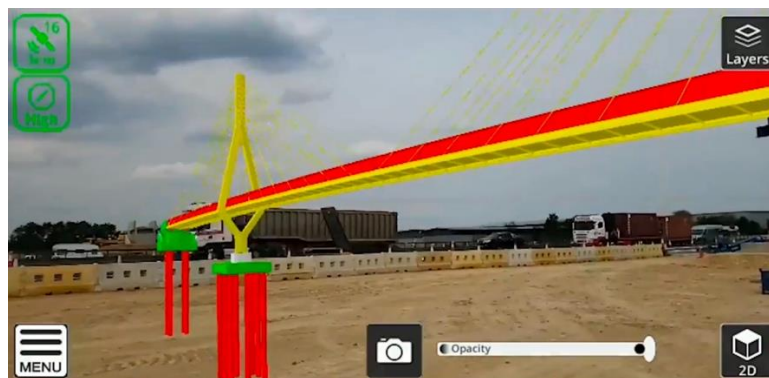
Figure 3: SiteVision visualization for the A14 Motorway Project
