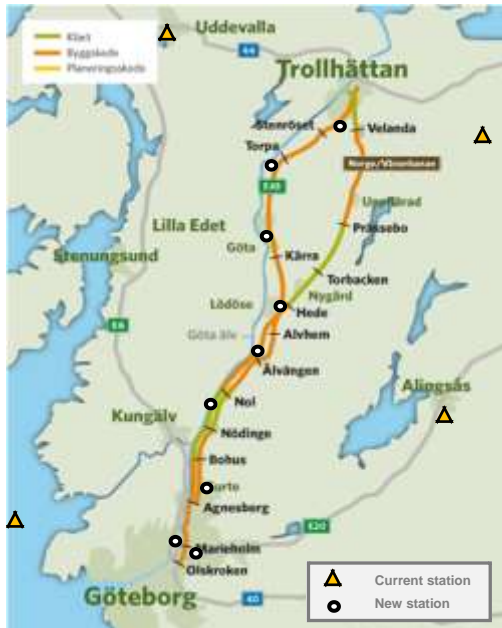
Figure 4, The Swepos network in the project area was densified by further 9 new reference stations in two stages for the PA-NRTK: Marieholm-Älvängen, and Älvängen-Trollhättan. The yellow triangles in the figure represent the Swepos stations when the project started. © Trafikverket.
