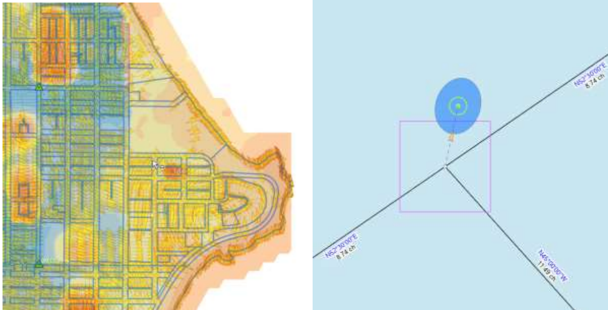
Figure 2: ArcGIS Pro advanced visualizations can be used to visualize LSA results such as Spatial Accuracy Heatmaps, error ellipses and outliers. (Data courtesy of Sheboygan County Wisconsin)
