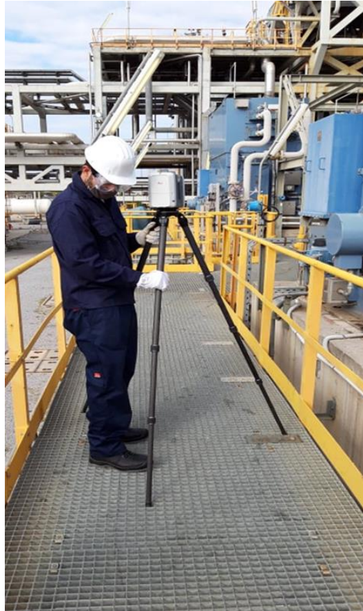
Figure 2 - Survey staff with RTC scanner in CCR area
