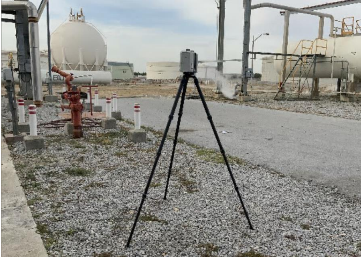
Figure 1 - The Leica RTC Laser Scanner in the area of Oil refinery
