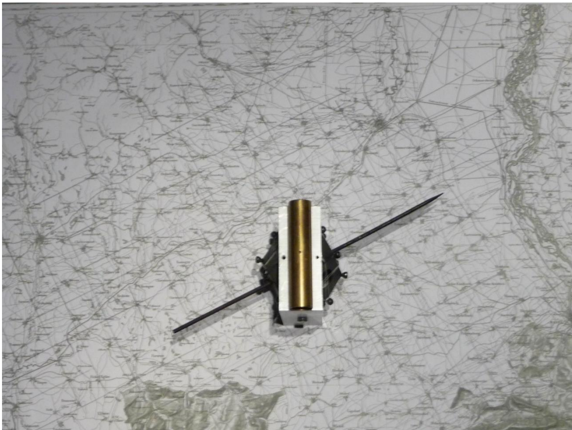
Fig 6: Positioning the axle of the starfindertube parallel to the axis of rotation of the dodecahedron will result in ENE-alignments of 63.435° from N .
