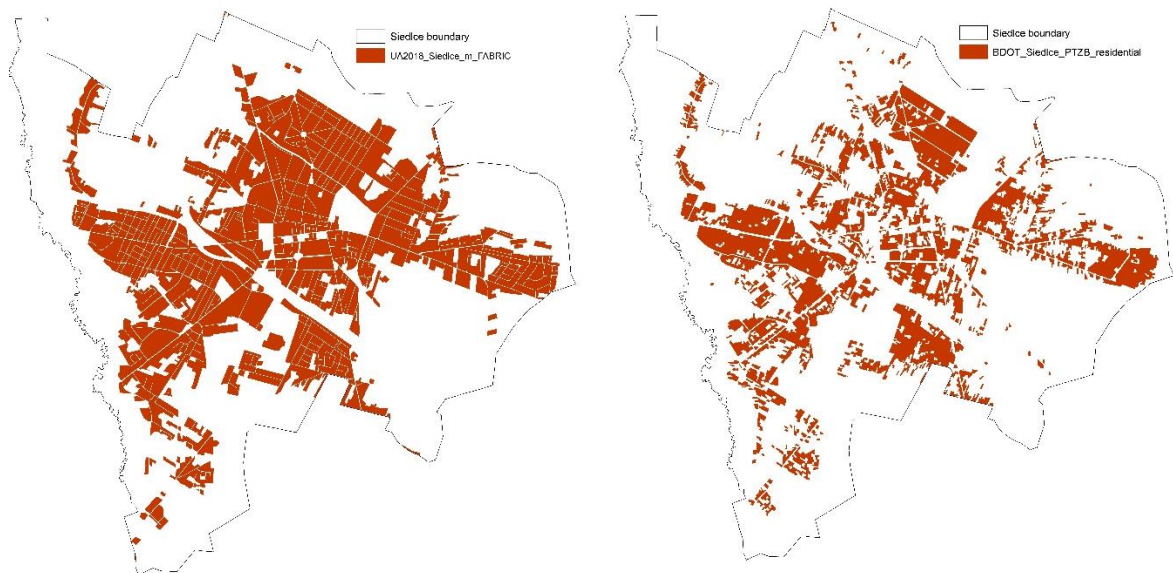
Figure 5 - Presentation of the regions where residential areas are found in the town of Siedlce. Left side: The urban fabric class from the Copernicus Urban Atlas map product. Right side: the reference BDOT10k residential areas class.
