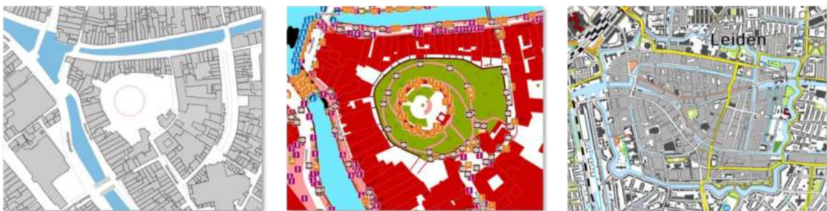
Figure 5: Key Register Addresses and Buildings (BAG), Key Register Large Scale Topography (BGT), Key Register Topography (BRT).
