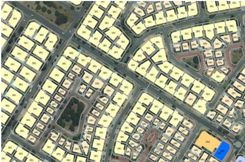
Figure 2: Single Residential and General Residential 2D DMS footprints illustrating the spatial extent of property RRRs using a 2D polygon, denoting the street and common boundary building setback lines.
