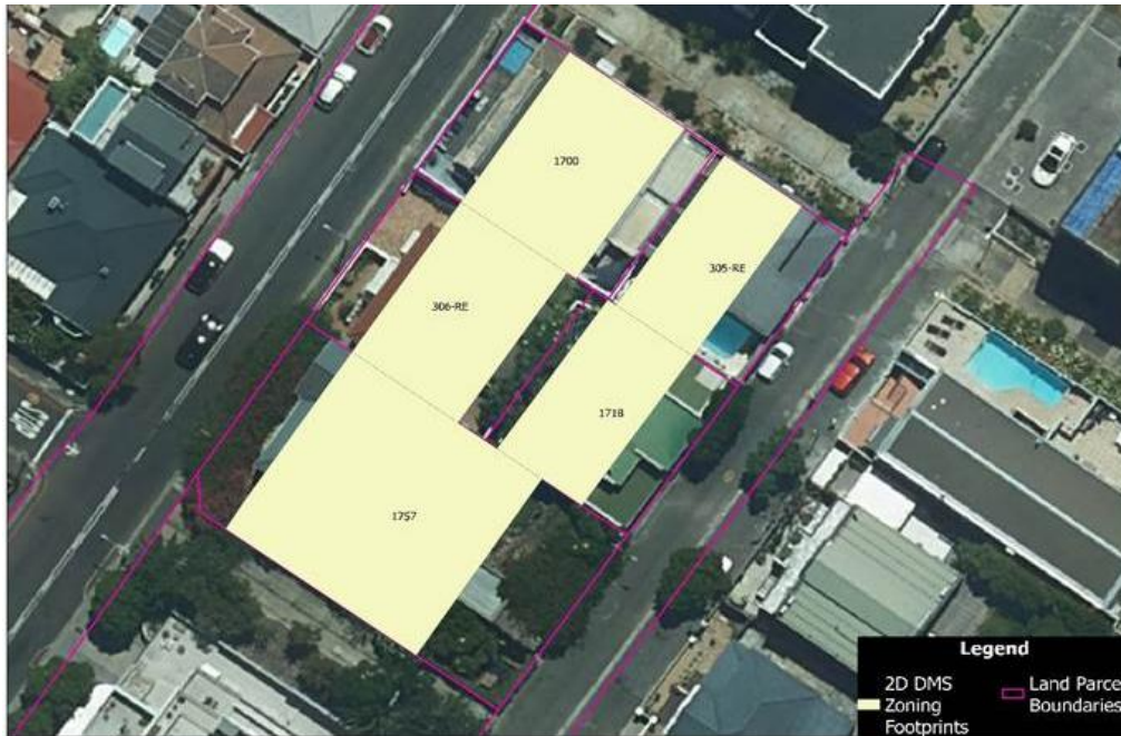
Figure 4: General Residential (GR4) 2D DMS footprints showing the spatial extent of property RRRs. The permissible developable area is defined with reference to street and common boundary building setback lines.
