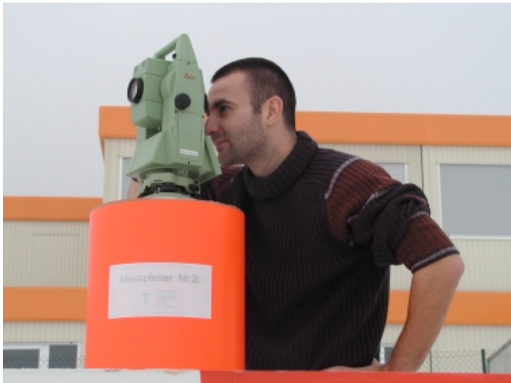
Fig. 1: Terrestrial measurements with the Leica TCRA 1103
