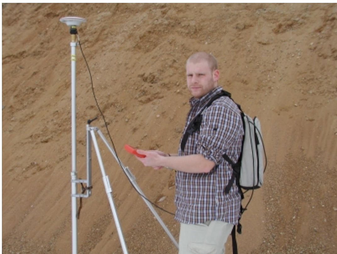
Fig. 2: Real-Time DGPS measurements with the Leica SR530
