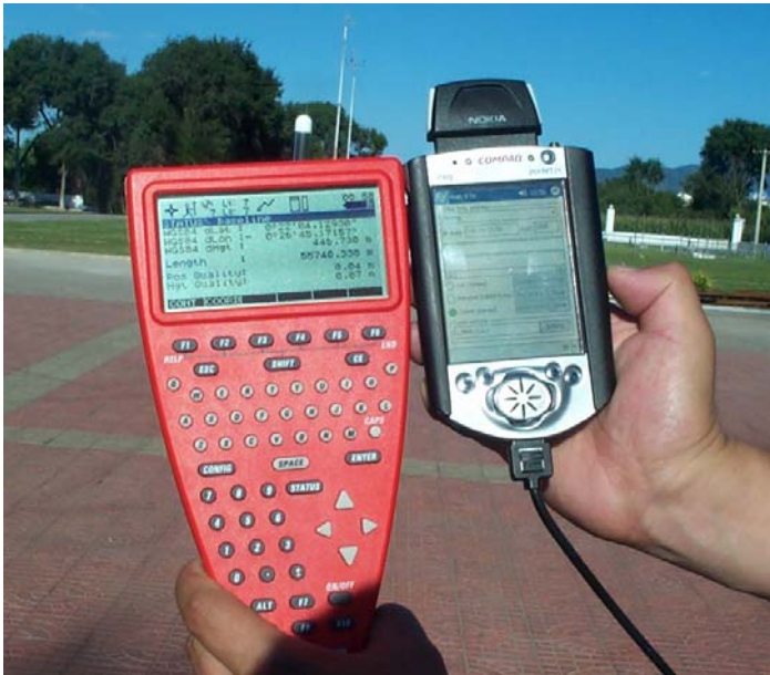
Diagram 7: RTK position fixed over Internet for 55740m baseline
