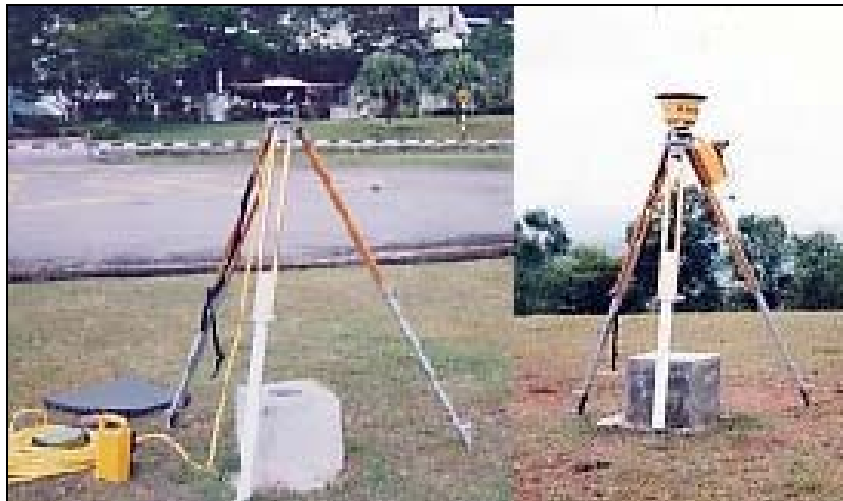
a) Ground Plane antenna b) Normal antenna
